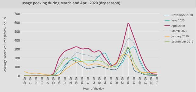
Figure 15: Quantity of water pumped at the Gajendrapur 'twin' tubewells showing usage peaking during March and April 2020 (dry season).
