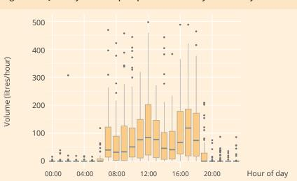
Figure 12: Quantity of water pumped from PSFs by time of day.
