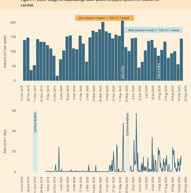
Figure 7: Water usage at Kapalidanga solar-powered piped system in relation to
