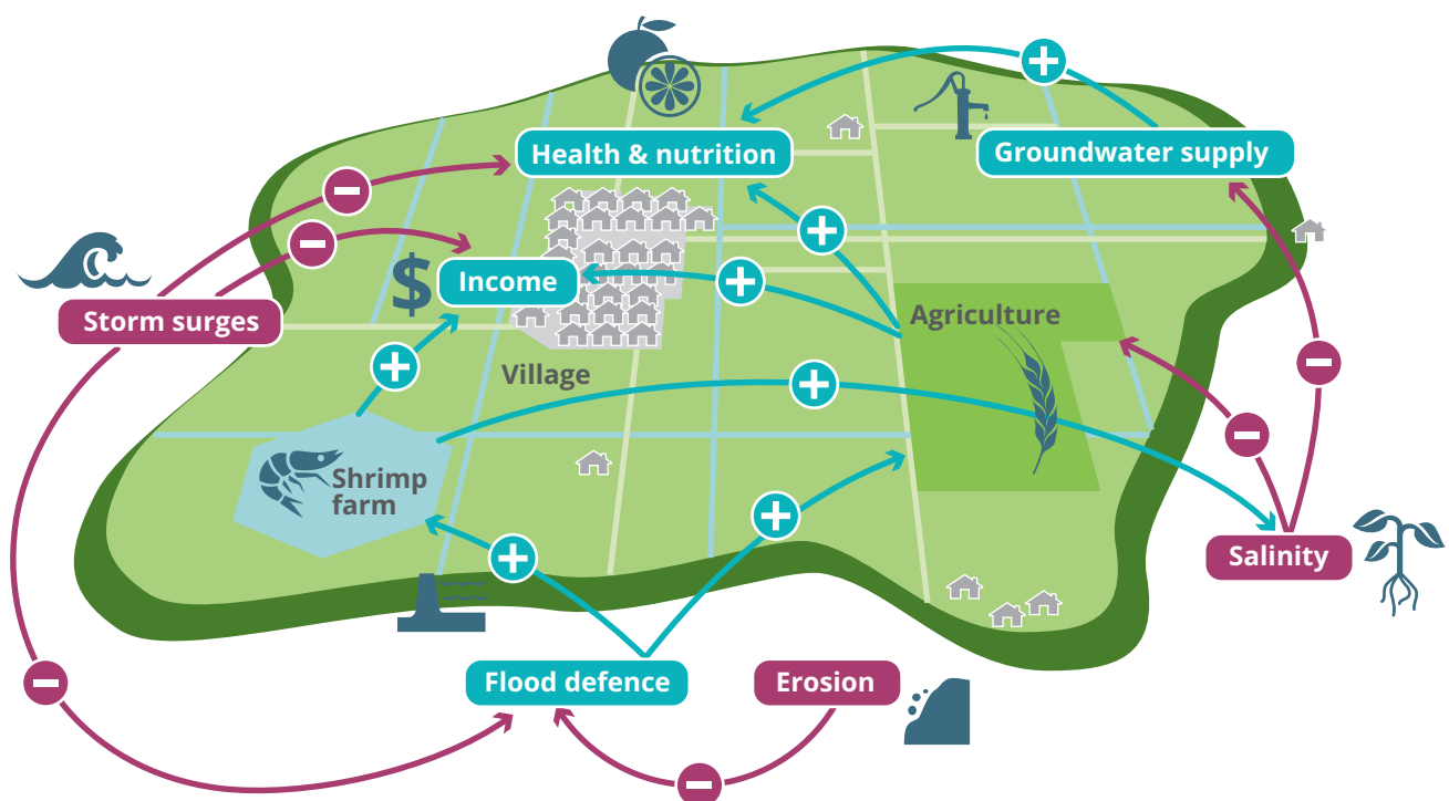
Figure 5: Schematic representation of a polder system showing interactions between hydrological, social and economic elements. For instance, the negative impact of salinity on agricultural production and groundwater supply (minus sign) reduces the positive impacts of agriculture on incomes and of safe groundwater supply on health (plus sign).
