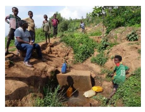
FIGURE 13. Measuring spring flow in Boloso Bombe *woreda* utilising a jerry can and mobile phone stopwatch. Photo from: David Walker.
