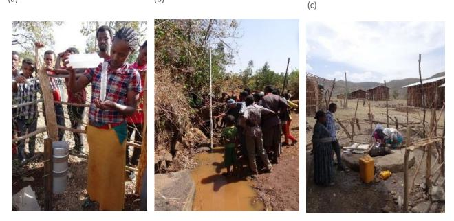
FIGURE 14. Observer training in Boloso Bombe and Ebinat woredas. (a) Rain gauge. (b) River staff gauge. (c) Dip-meter. Photos from: David Walker.
