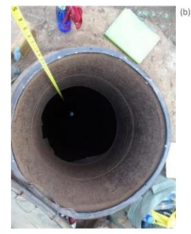
FIGURE 12. (a) and (b) Measuring groundwater levels in hand-dug wells in Boloso Bombe *woreda*. Photos from: David Walker.
