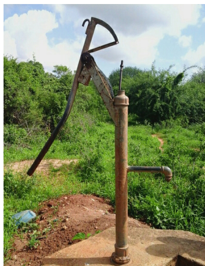
Tany and Tara handpumps are few compared to the Afridev type but record higher non-functionality rates in Kitui (Photo Credit: Cliff Nyaga/Oxford University)
