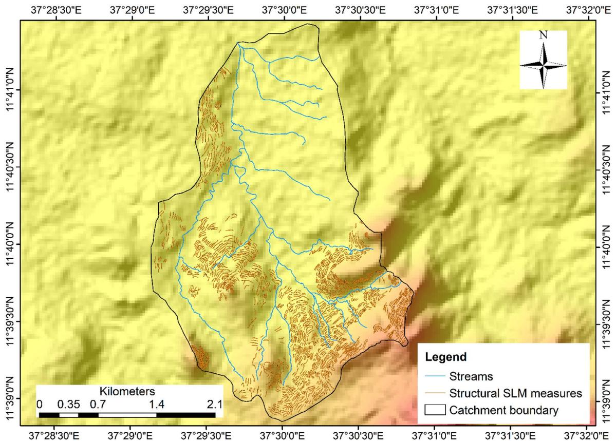
**Fig. 2** Distribution of structural SLM measures (soil bunds; contour trenches) in the treated Aba Gerima catchment
