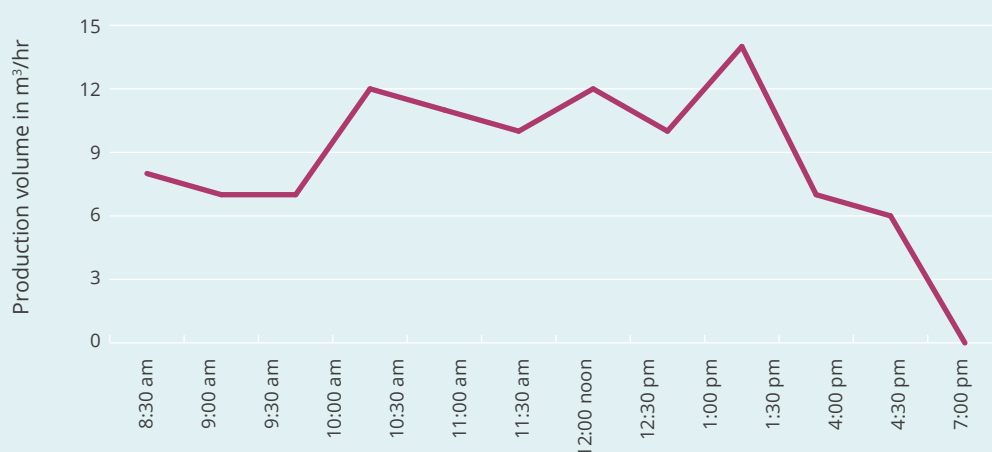
Figure 24: Daily variation of borehole production (m 3 /hr) in a Lodwar Water Supply and Sanitation borehole, Kenya. The figure indicates that water availability depends on the energy source used in pumping, with erratic pumping observed in boreholes using solar energy. Source: Maxwell et al. (2020).
