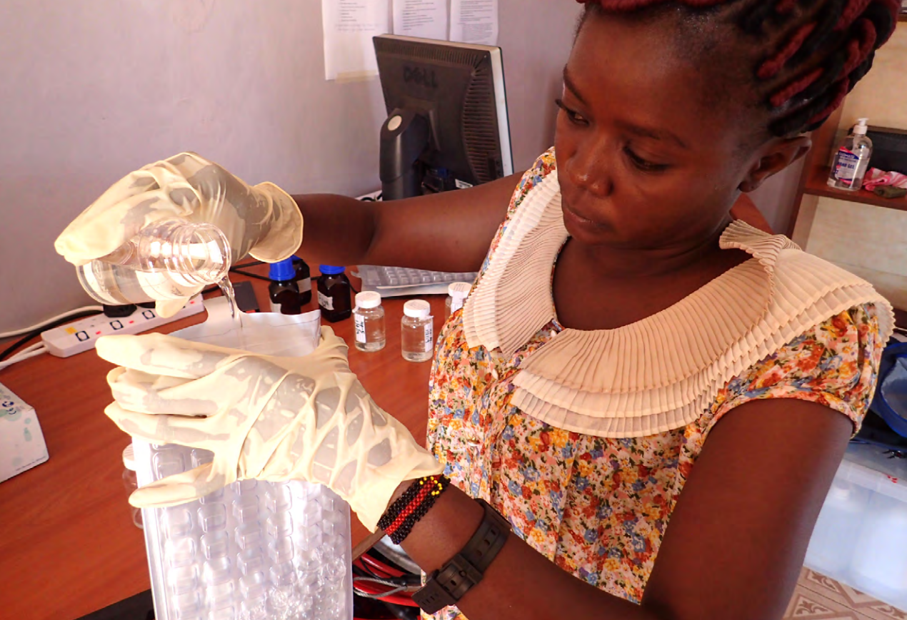
Mary Musenya Sammy, FundiFix water quality officer, preparing a sample for E. coli analysis in the field lab in Kyuso, Kitui. Credit: Saskia Nowicki
