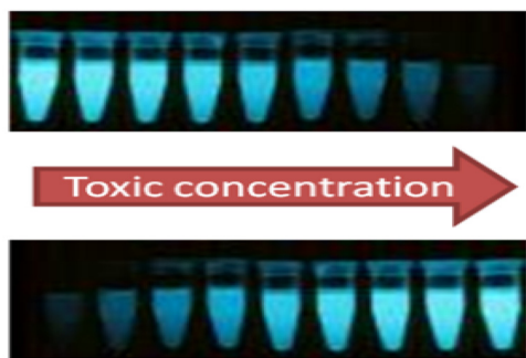
Fig. 4. Luminescence from the bacterial biosensors reflecting cyto- or geno toxicity.
