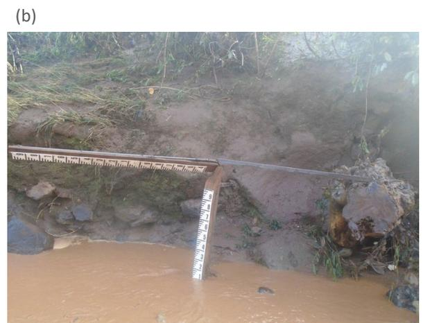
FIGURE 5: Substantial maintenance of monitoring equipment in Ethiopia. (a): Repairing the base and fence of a raingauge. (b): A river staff gauge requiring reconstruction following damage by floating debris during a flood. Photos from: David Walker and Dawit Bunduro.
