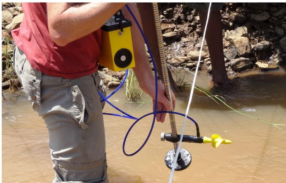
FIGURE 2: An impellor current-meter in use for flow gauging in Ethiopia. Photo from: David Walker.
