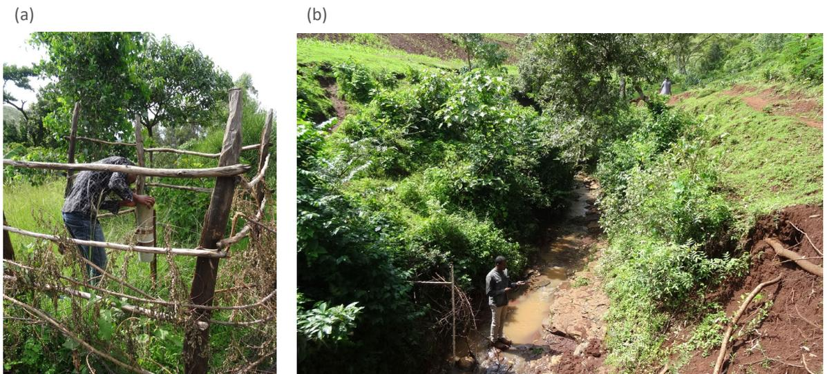
FIGURE 4: Minor maintenance of monitoring equipment in Ethiopia. (a): Cleaning a raingauge and removal of tall obscuring grass. (b): Clearing debris (a tree branch) from a river staff gauge. Photos from: David Walker.
