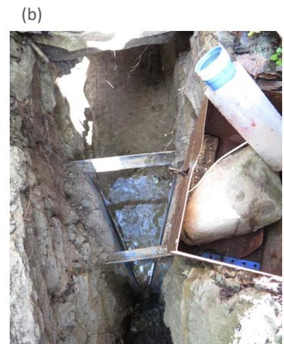
FIGURE 10: A weir and a flume for monitoring flow. (a): A combined v-notch (for low flows) and rectangular weir (for higher flows) in South Africa. (b): A 30 mm flume within a stone-lined channel above a spring in India; flow is from top to bottom of the photograph. Photos from: David Walker.
